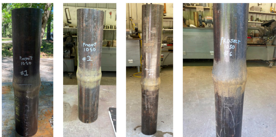
Example of test pipes expanded using various charge sizes
